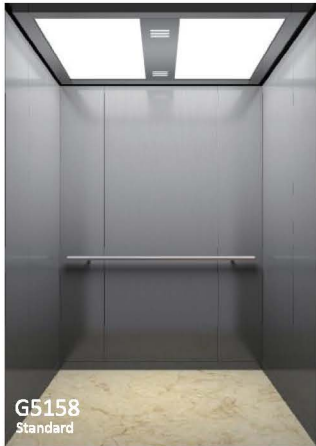
G5158 Standard Ceiling: Hairline stainless steel, white acrylic + LED (G1008) Cabin panel: Hairline stainless steel COP: Hairline stainless steel (G2116) Handrail: Round hairline stainless steel (G6001) Flooring: Marble (G3308)
