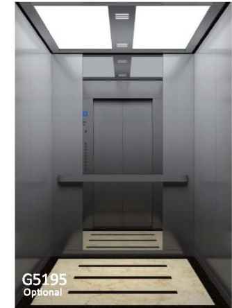
G5195 Optional Ceiling: Hairline stainless steel, white acrylic + LED (G1008) Cabin panel: Hairline stainless steel Mirror Stainless Steel COP: Hairline stainless steel (G2116) Handrail: Hairline stainless steel (G6003) Flooring: Marble (FT-06)
