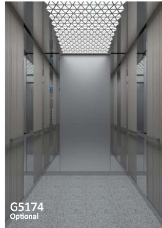
G5174 Optional Ceiling: Mirror stainless steel, white acrylic + LED (G1045) Cabin panel: Brushed Stainless Steel Mirror Stainless Steel Composite Board (G4330) COP: Hairline stainless steel (G2116) Handrail: Round hairline stainless steel (G6011) Flooring: Marble (G3313)
